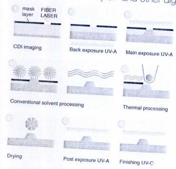
The digital flexo plate has a mask layer – sensitized to the CDI's laser light – on top of its surface. After imaging, this mask takes the function of the traditional film negative. Through the integration of the image carrier, a digital flexo plate has sharper absorption and scattering in the traditional contacting through vacuum sheet and film is totally eliminated.
